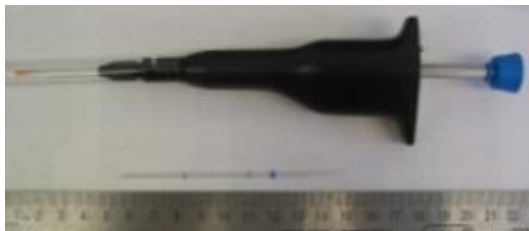
Figure A5. 100 \mu L Drummond Micro Pipetter (top) and tip (bottom) with ruler for scale.
