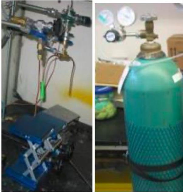
Figure A6. Ultra-pure Nitrogen tank (Right) and Nitrogen blowdown station (Left).
