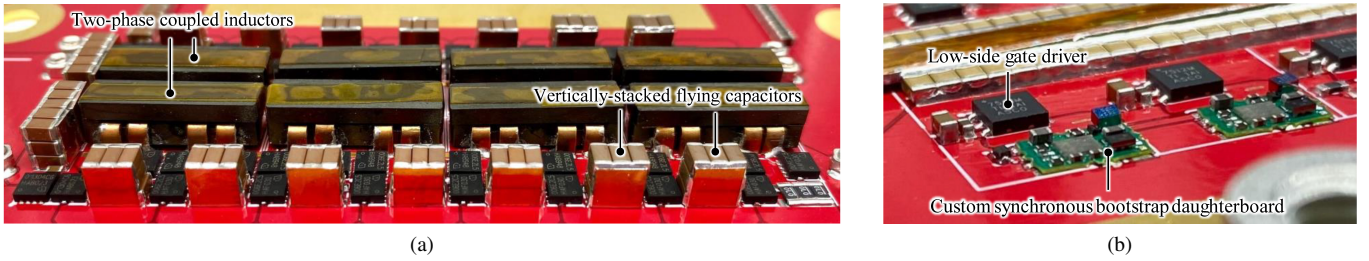
Fig. 10: (a) Side view of the hardware prototype. (b) Photograph of the gate drive circuitry, including the custom synchronous bootstrap daughterboards (dimensions: 5.8 \times 3.5 \times 1.0 mm 3 ) used to power the high-side switches.
