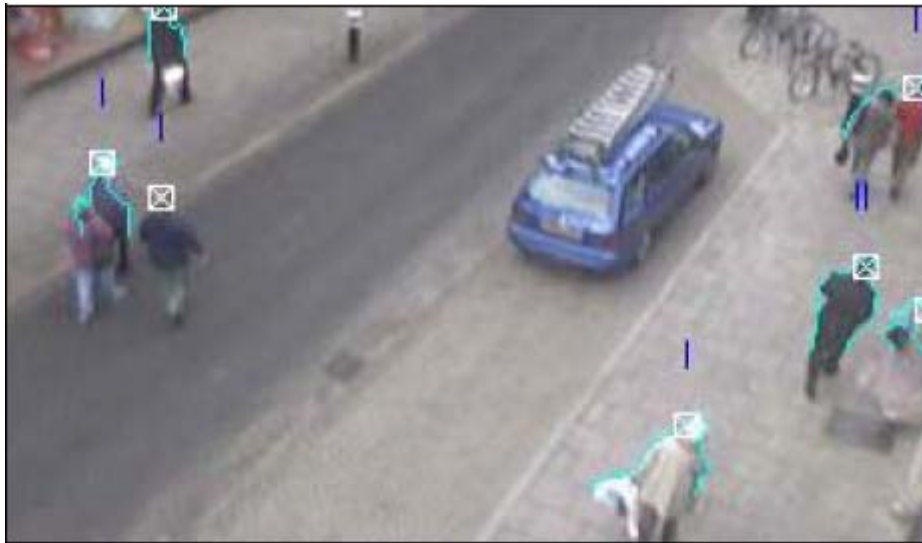
Figure 4.4: Video Imaging for Counting Pedestrian (CLP, 2005)
