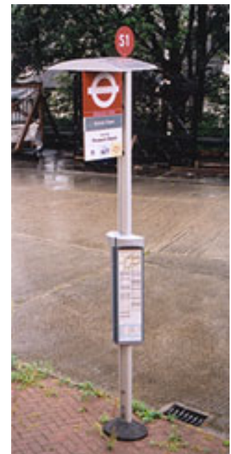
Figure 20 Solar-powered beacon and illuminated schedule display (left and center) and solar-powered light to illuminate existing sign and schedule display
