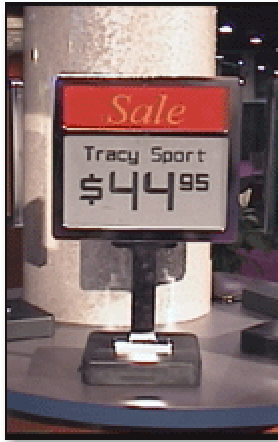
Figure 22 Sign Using SmartPaper
