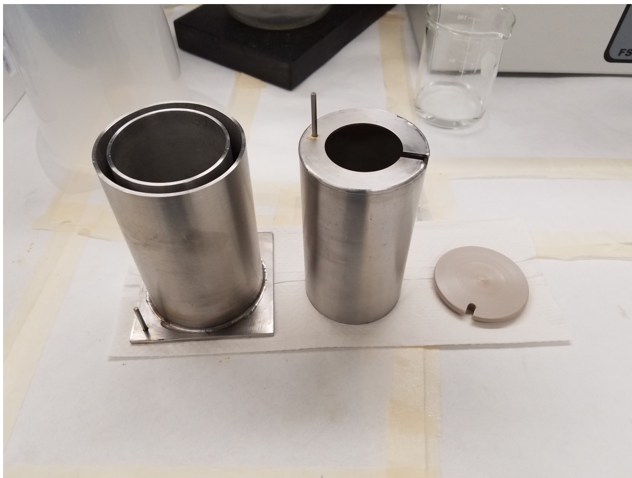
Figure 2.2: The liquid capacitance cell is shown disassembled. Fluid is held within the cylindrical shell to the left. The middle cylindrical piece slides between the gap of the shell, making a capacitor. The two metal parts are all solid constructions. The PEEK spacer is shown to the right
