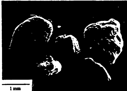
Fig. 2. Collection of typical conditioned quartz particles used in fluidized bed wear study.
