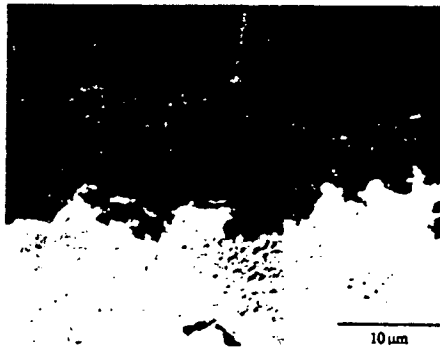
Fig. 7. Optical micrograph of surface cross-section from the 0° rod location of the 6061-T6 specimen from Task 2 showing deposit layer on surface.
