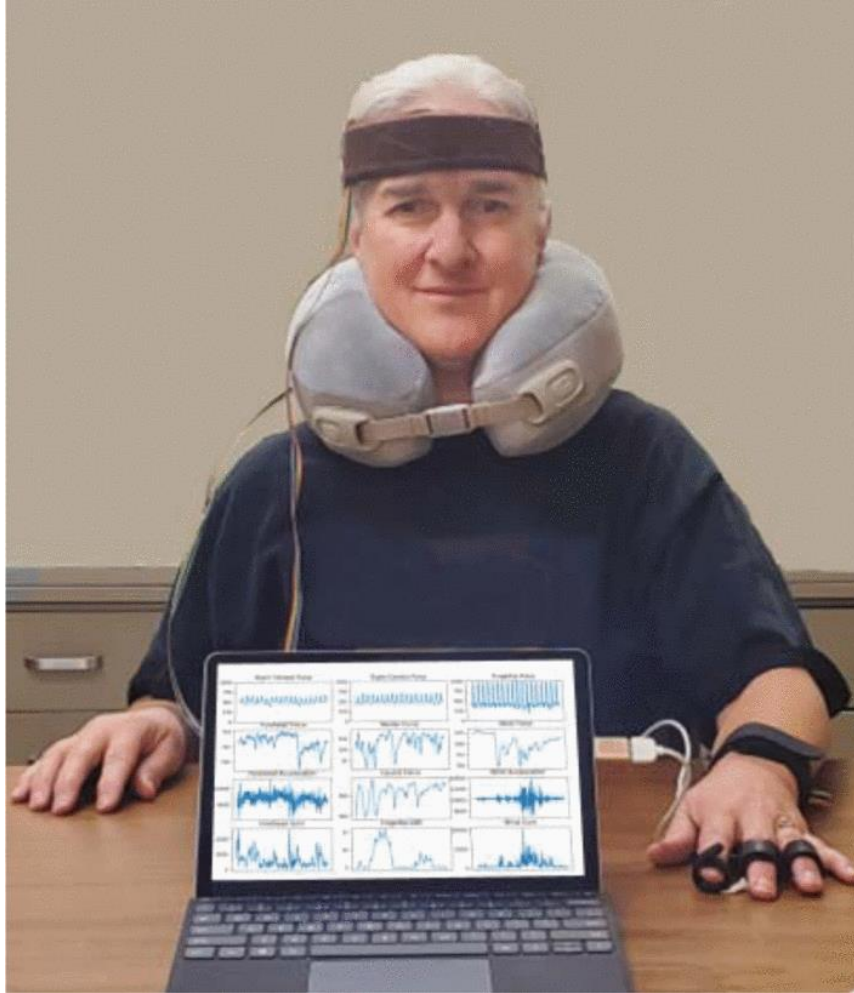
Figure 9. Pain meter 2 consists of: 1) PPG pulse sensors in a headband, in a neck band, and on the fingertip, 2) Temperature sensors on the neck and fingertip, 3) 3-axis accelerometers and 3-axis gyros in the head band and wrist band, 4) Force sensors on the forehead, back of neck, side of neck, and wrist band, and 5) GSR sensors between the middle and ring fingers.
