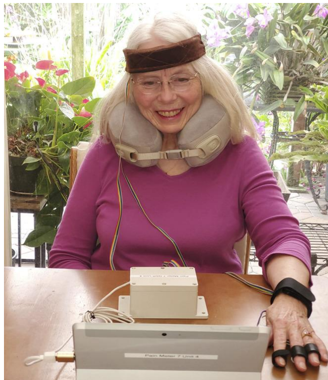
Figure 23. Pain Meter contains (1) PPG pulse sensors in a headband, in a neck pillow, wristband, and on the fingertip; (2) temperature sensors on the temple, forehead, wrist, and fingertip; (3) 3-axis accelerometers and 3-axis gyros in the headband and wristband; and (4) force sensors on the left carotid and basilar. PPG, photoplethysmograms.
