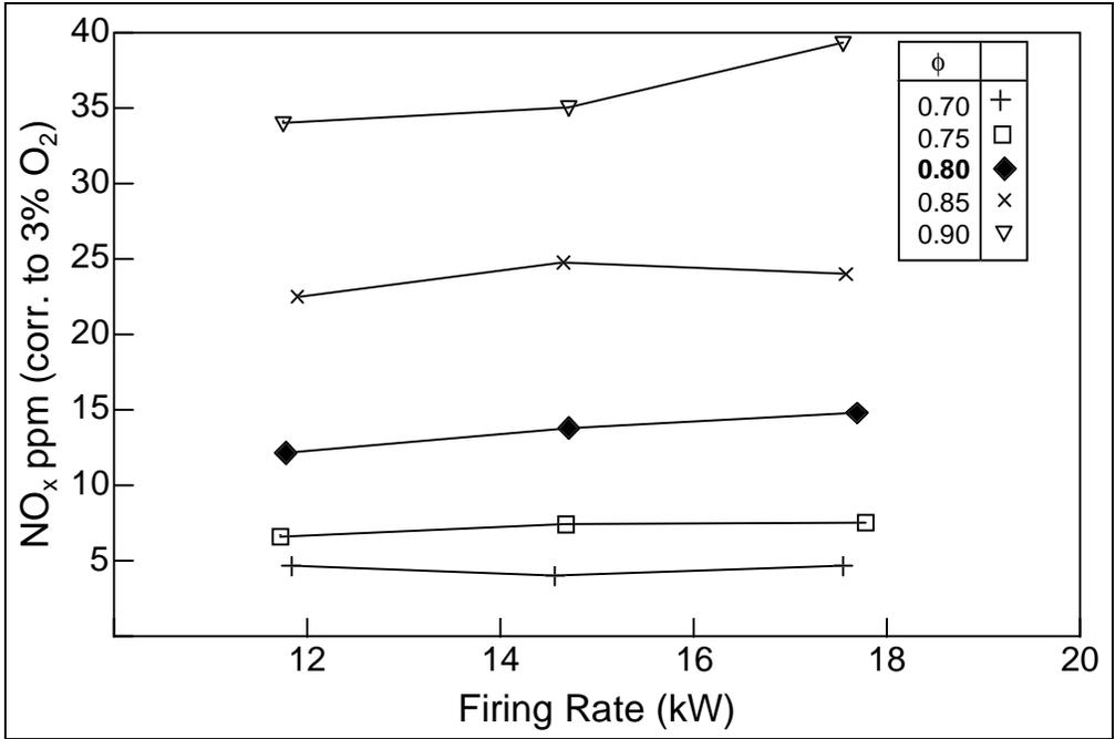
Figure 5:  $\text{NO}_x$  emissions from the LBNL water heater simulator with the 5 cm WSB ( $A_c / A_b = 15$ ) displays primary dependence on the equivalence ratio and little dependence on firing rate. For  $\phi < 0.90$ , the WSB exceeds the strictest regulations of SCAQMD 1146.2
