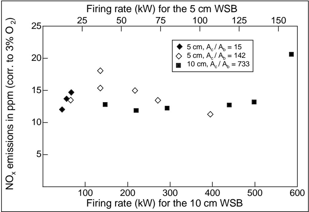
Figure 7: NO<sub>x</sub> levels are constant at ≈ 15 ppm for the three chamber/burner ratios and for a firing rates from 12 to 585 kW.
