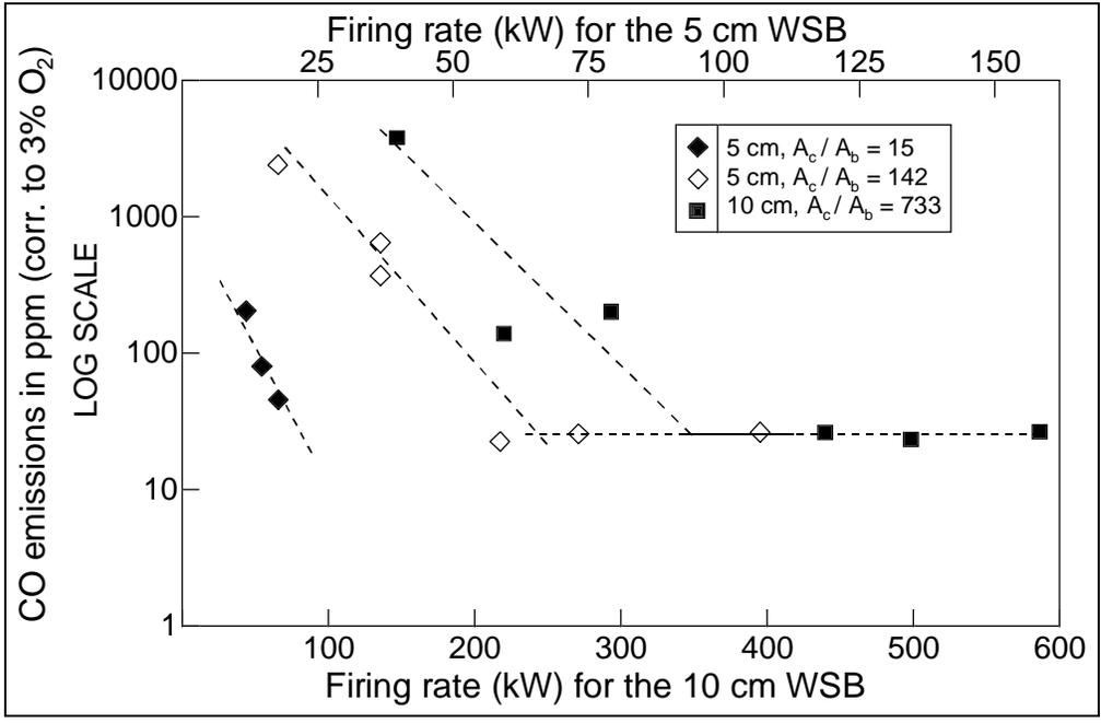
Figure 8: As plotted on a logarithmic scale, CO emissions display a strong dependence on both firing rate and  $A_c/A_b$ . Minimum firing rates of ≈ 25, 65, and 400 kW are necessary to achieve CO levels of 25 ppm for  $A_c/A_b = 15, 142,$  and  $733$  respectively. Dashed lines are not fit to the data.
