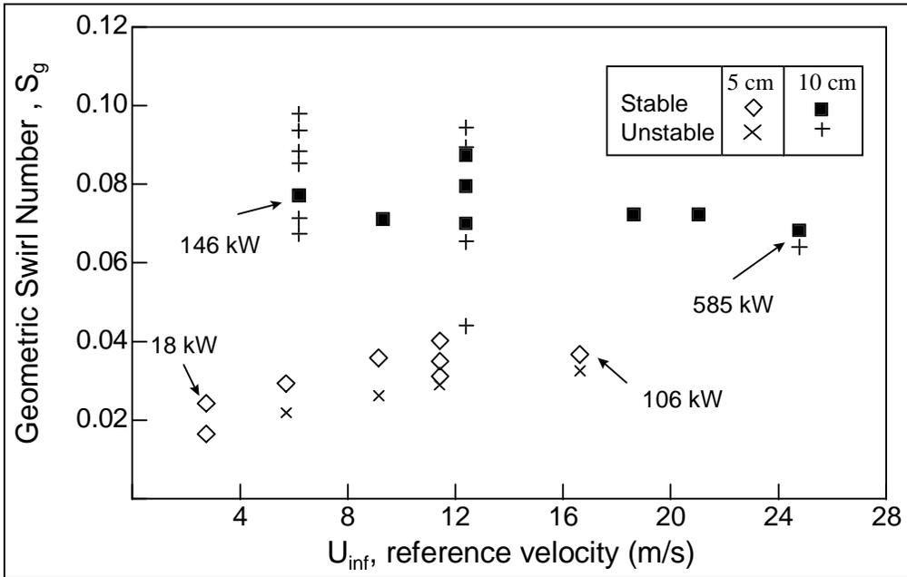
Figure 4: The operating regime of the 5 and 10 cm in the UCICL combustion chambers over similar velocity regimes shows a significant increase in the non-dimensional swirl number  $S_g$  (and thus swirl air) needed for stability.
