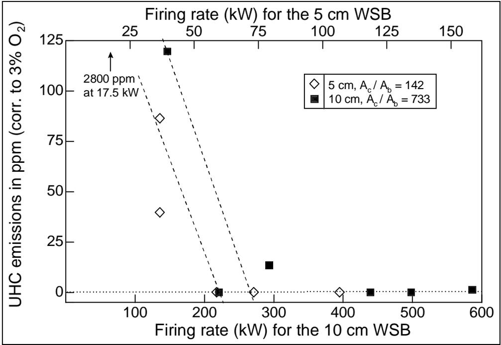
Figure 9: UHC emissions decrease dramatically with increasing firing rate however no conclusion can be drawn on the effect of  $A_c / A_b$  on emission levels. Above  $\approx 75$  and 300 kW (similar  $U_{ref}$  of 12 m/s), emissions are essentially 0 ppm.
