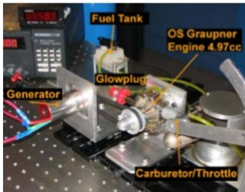
Figure 45: Experimental setup with a throttle control, belt driven dynamometer and manual
