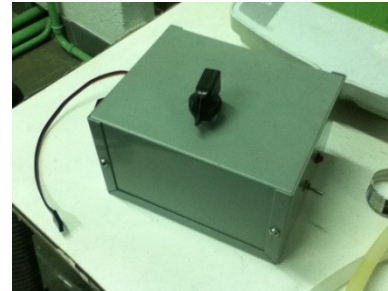
Figure 102: The bulky box that contains a potentiometer to drive the PWM signal to any standard hobby signal. This solution was replaced by ArduinoUNO micro controllers upon their discovery.
