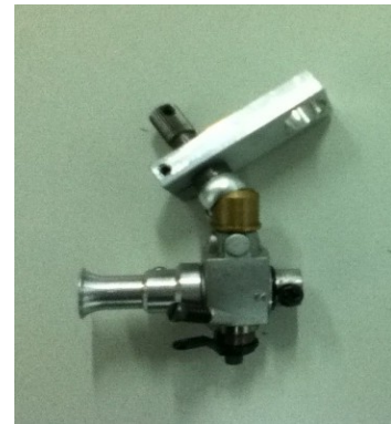
Figure 106: O.S. Graupner Wankel carburetor with angular encoder mount.
