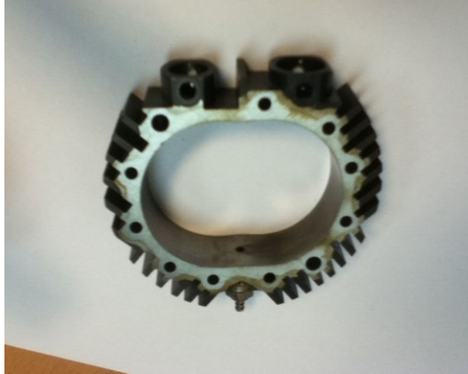
Figure 95: This image illustrates that no new chamber pockets / ports were drilled unnecessarily creating more unwanted dead volume (as in Cardes et al [93]). This was achieved with the help of the technical staff at the Universidad Politécnica de Madrid.
