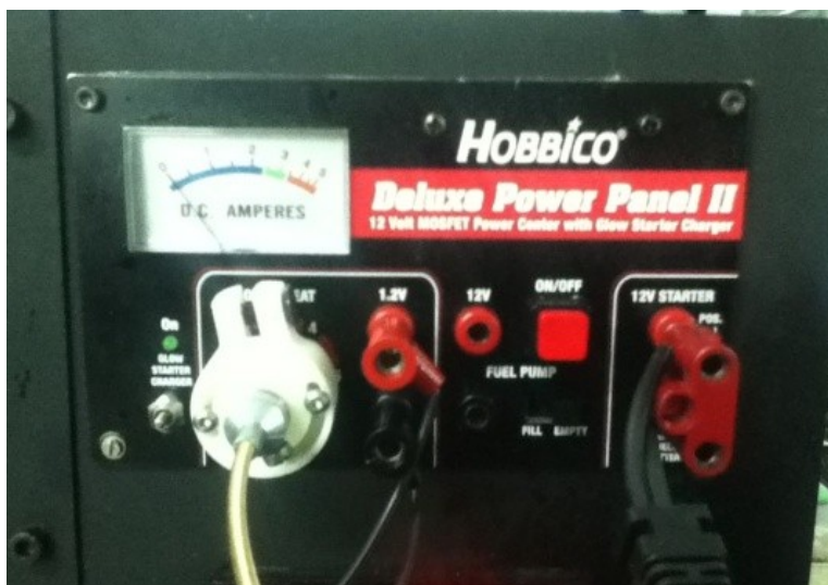
Figure 112: The Hobbico Deluxe Power Panel which helps manage power delivered to the glowplug and starter motor.
