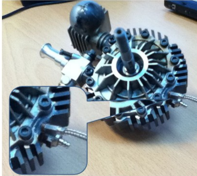
Figure 97: A magnified view of the rotary engine with the Optrand Auto-PSI high temperature pressure sensor installed.
