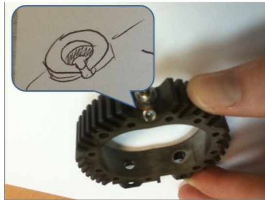
Figure 96: This image attempts to show the landing surface for the pressure sensor. The dull brown ring is the crush washer for the glow plug, and the horseshoe shape is the flat surface landing for the sensor. However, the mouth of the horseshoe illustrates a leakage point for combustion gases and needs to be sealed.
