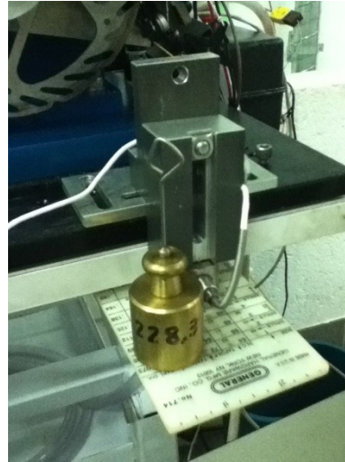
Figure 164: Here the load cell is being pulled in tension. The screw thread checker is being used as a plate to support the calibration weights.
