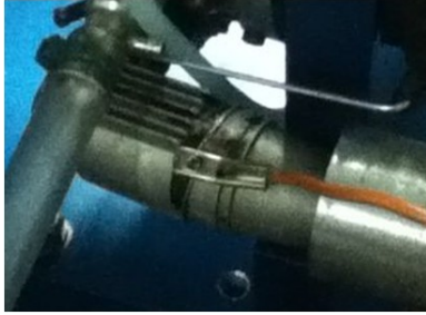
Figure 149: Exhaust thermocouple position.
