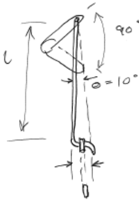
Figure 103: Linear to rotary motion of throttle servo mechanism (top view).
