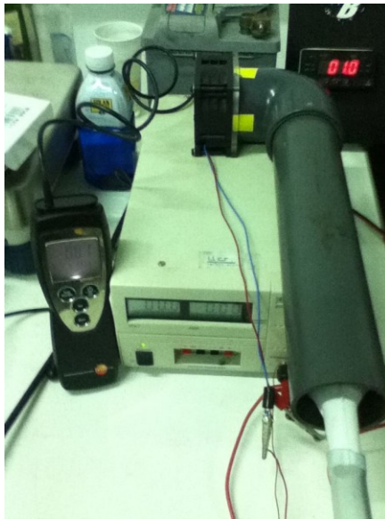
Figure 169: Left most sensor is the Testo 425 air anemometer. Middle is a 75W 30V power supply, Above the power supply is the calibration unit.
