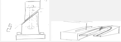
Figure 93: Design sketches load cell sensor mount with focus on adjustability.
