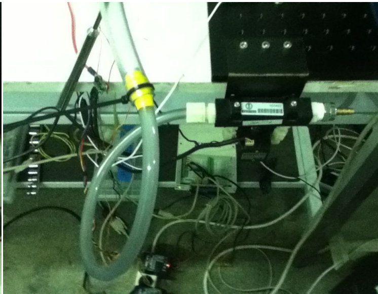
Figure 170: The Testo 425 probe enters the air flow tube at the top of the photo. The tube continues on into the sensor being calibrated.
