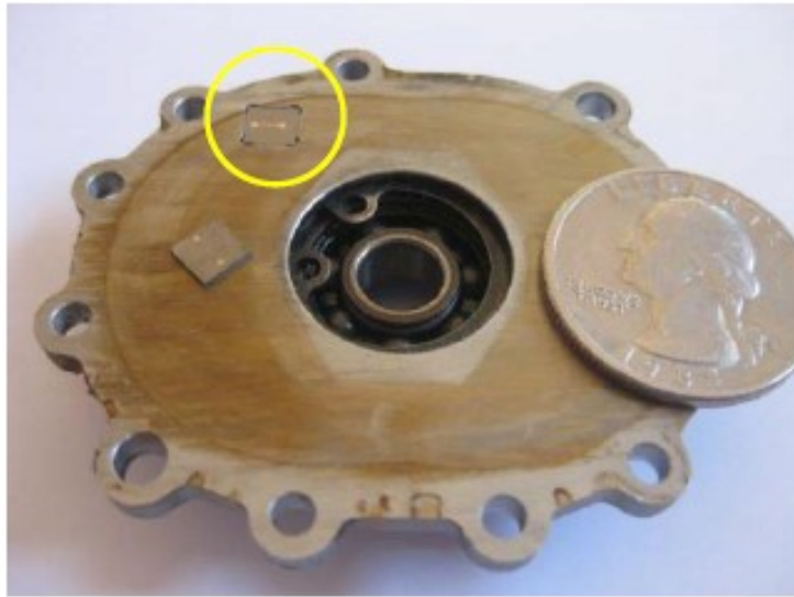
Figure 23: A MEMS-based temperature sensor designed and fabricated by S. Wodin-Schwartz is embedded into a 4.97 cc Wankel Engine by C. McCoy to test survivability of MEMS devices in real combusting small-scale engines [43]. The circle identifies the location 5 \times 5 \text{ mm}^2 pocket for the MEMS temperature sensor.
