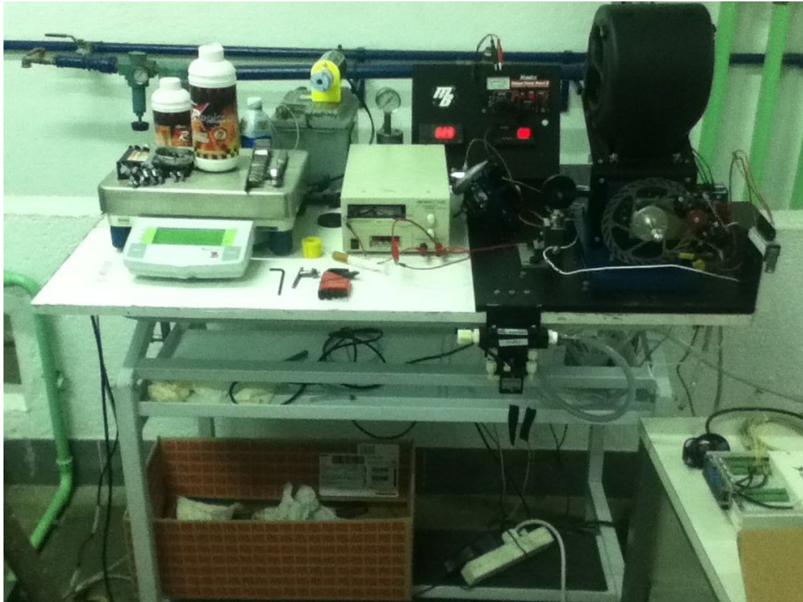
Figure 78: The fuel-flexible rotary engine testing setup at the Escuela Técnica Superior de los Ingenieros Aeronáuticos (E.T.S.I.A.), an aeronautical engineering school that is part of the larger polytechnic university (la U.P.M.) in Madrid, Spain. With a larger engine lab and more equipment available for the characterization of engines, the dynamometer characterization system was set up and modified to continue testing in this university. The primary modifications and tools used were the mechanical loading system, fuel switching system and the emissions measurement equipment.
