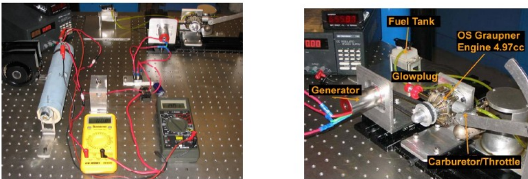
Figure 125: Left: testing dynamometer for the O.S. Graupner Wankel Engine. Right: Close-up view of generator and test stand [93].
