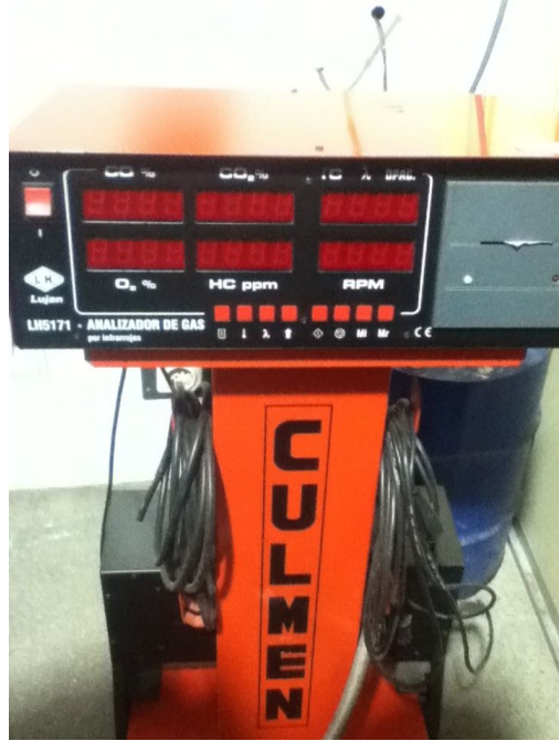
Figure 90: The Lujan emissions measurement system. This system was designed for auto emissions and was expected to potentially yield strange results as other similar systems (like Horiba) were specifically designed for automobile-scale emission volumes.
