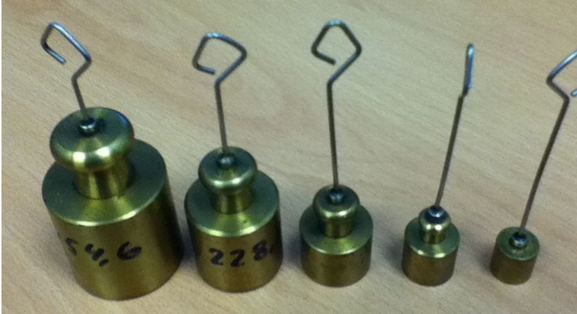
Figure 165: Calibration weights used to calibrate the Sensotec load cell and compare Ohaus Explorer precision mass balance.
