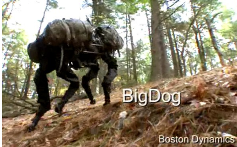
Figure 10: The BigDog from Boston Dynamics has an impressive ability to carry payload and handle complex terrain. Its current powertrain is a very noisy, 2-stroke, 15hp engine [21].
