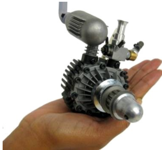
Figure 71: The small-scale O.S. Graupner Wankel engine with an engine displacement of 4.97 ccs. Hand model credit goes to Dr. Debbie Senesky.
