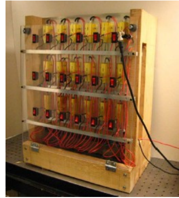
Figure 85: The final assembly of the resistor bank. The high power resistors are mounted directly to the heat sink with cooling fans (not visible from this photo)
