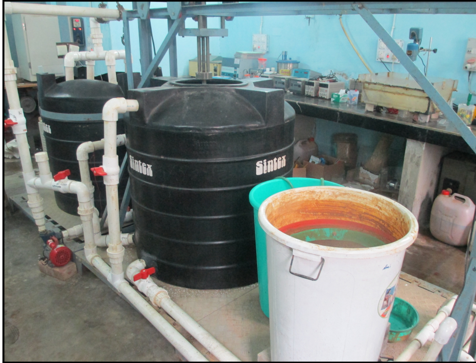
Figure 1.3: 700 L electrocoagulation field prototype in Kolkata, India (Photo: C. van Genuchten)
