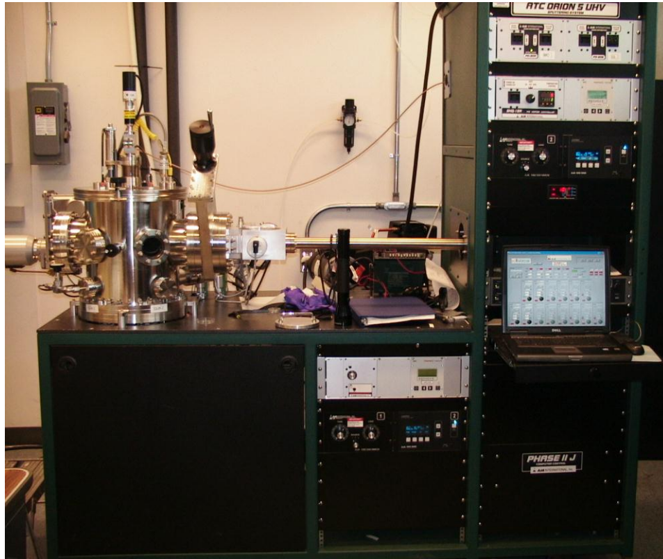
Figure 44. The ATC ORION 5 UHV Sputtering System used for SiO 2 film deposition.
