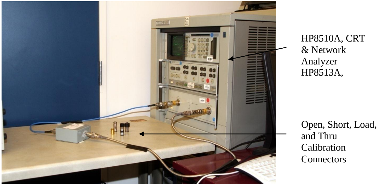
Figure 36. Network Analyzer Experimental Test Setup.
