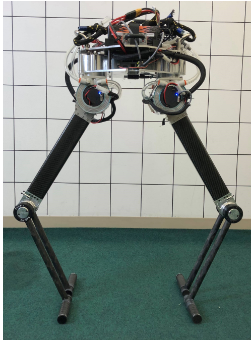
Figure A.1: NABi-V2 version robot added yaw DOFs at the hip joint [6].
