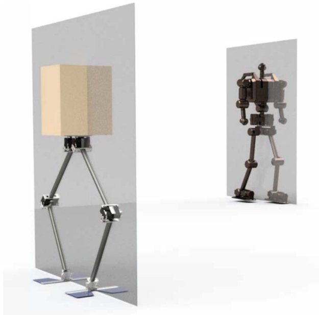
Figure 2.1: NABiRoS version robot showing rotation of legs in the sagittal plane when compared to a “typical” humanoid robot [1].
