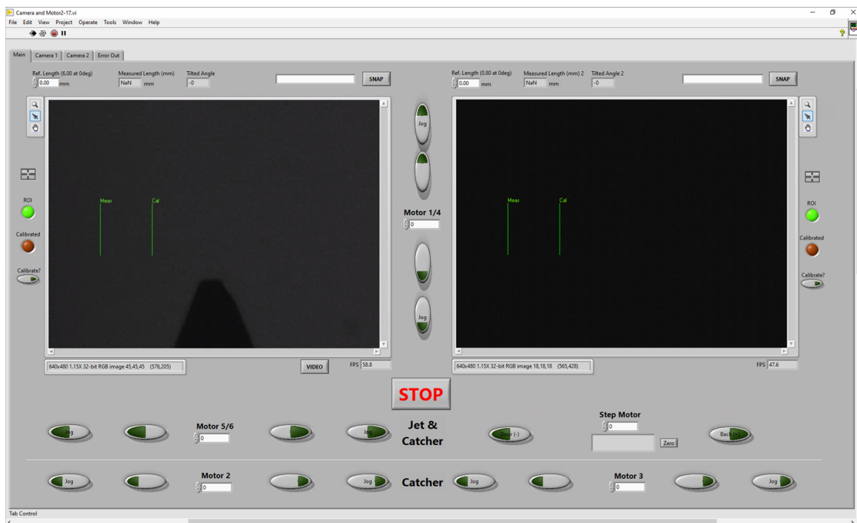
Figure B.1: Main page in the front panel of the liquid jet monitoring LabVIEW program. This is the main panel to control the jet position and monitor the jet status.
