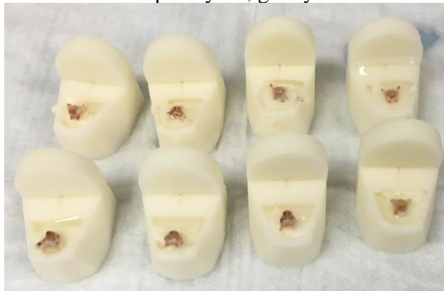
Figure B.15 – Mouse lumbar vertebrae with posterior processes potted in PMMA
