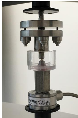
Figure B.22 – Experimental set-up with spherically-seated upper platen, lower platen, water-bath, and load cell all in place. Water-saline solution has not been added yet.
