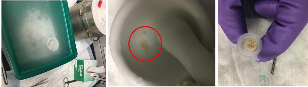
Figure B.30 – Bone crushing set-up. (Left) Containment ice bucket housing the mortar and pestle with liquid nitrogen to keep cold. (Middle) Mortar and pestle with crushed sample highlighted in red. (Right) Bone powder scraped into microcentrifuge tube using spatula.
