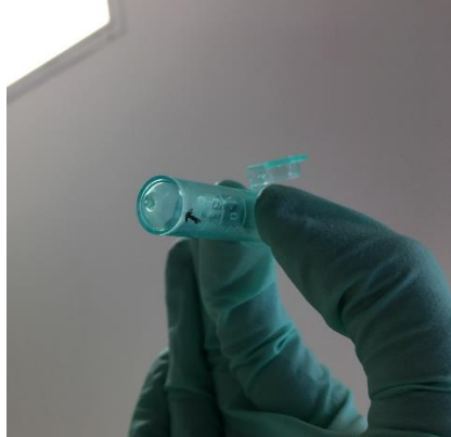
Figure B.32 – Pellet is sometimes difficult to identify. Hold sample under light and look for cloudy substance at the bottom rim of microcentrifuge tube. Black arrow drawn on tube to show where the pellet is located.
