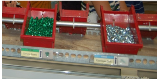
Figure 4: Color-coded Screws (and Corresponding Bin Labels) are Easy to Match/Tell Apart (facilitate recognition) (Source: Iris Tommelein)
