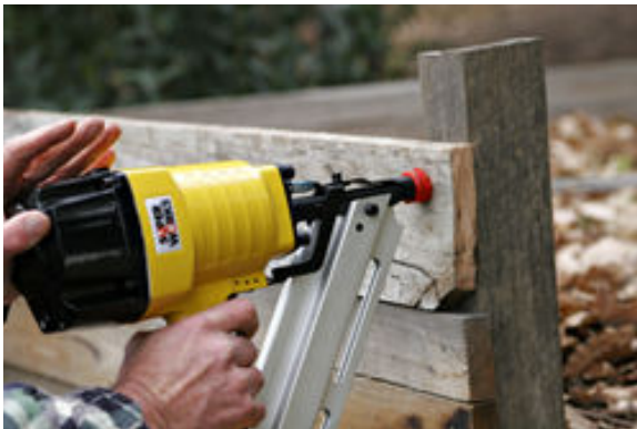
Figure 2: Pneumatic Nail Gun in Use ( en.wikipedia.org/wiki/Nail_gun )
