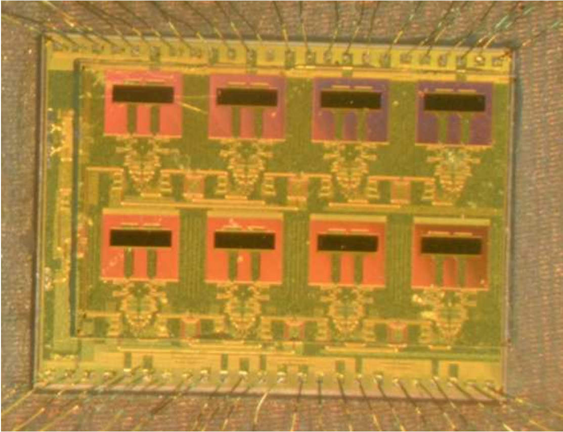
Figure 2.20: CMOS PA chip-quartz antenna wafer assembly wire-bonded to PCB mounted on copper block.
