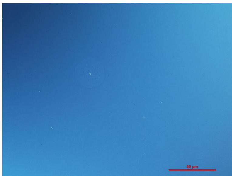
Figure 57. Optical micrograph of a corrosion feature on the \text{CrN}_x adhesion layer mirror after 6 months of laboratory storage. Note the difference in scale from previous micrographs of this mirror type.
