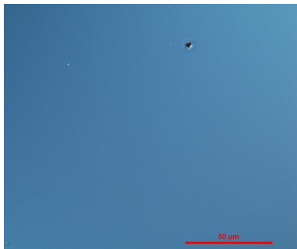
Figure 95. Optical micrographs of a corrosion nodule on the NiCrN x adhesion layer mirror after 10 days of MFG exposure.
