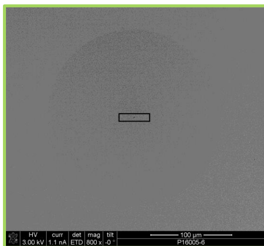
Figure 28. Plan-view SEM micrograph of a circular corrosion region on the CrN x adhesion layer mirror showing the location of the TEM cross-section. Reprint of Figure 19.
