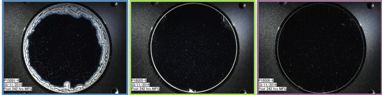
Figure 14. Dark field images after 10 days of MFG exposure of the no adhesion layer mirror (left), CrN x adhesion layer mirror (center), and NiCrN x adhesion layer mirror (right).
