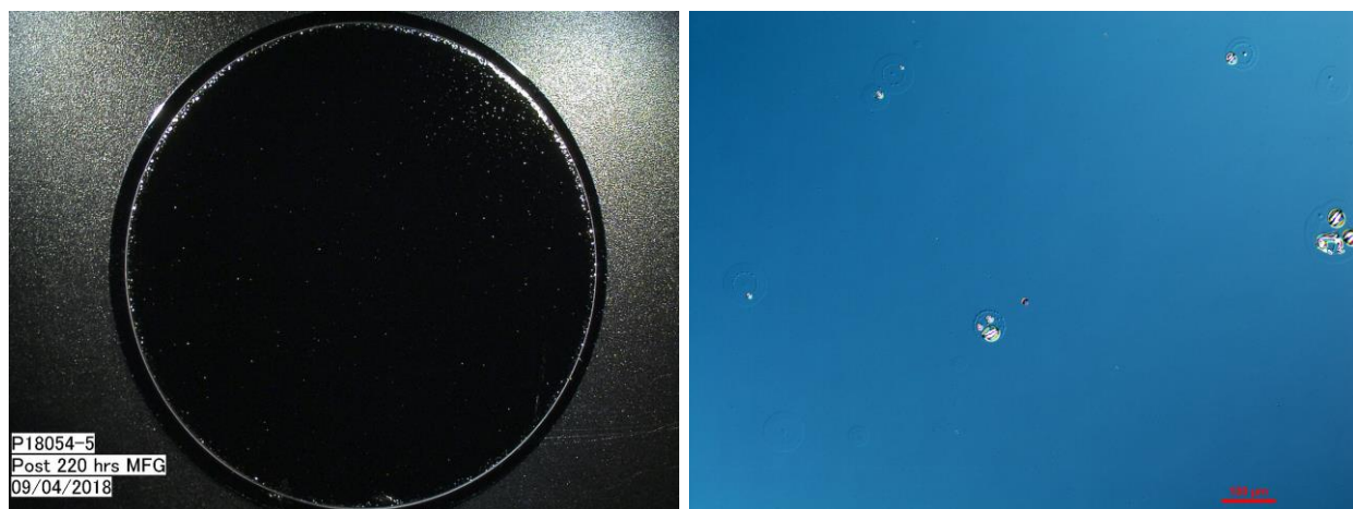
Figure 48. Dark field image of a Cr base layer mirror with corresponding optical micrograph of corrosion features after 10 days MFG exposure.
