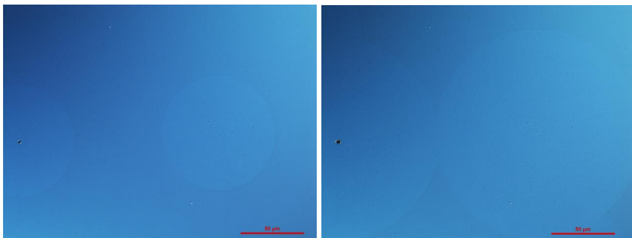
Figure 93. Optical micrographs of circular corrosion regions on the \text{CrN}_x adhesion layer mirror after 5 days (left) and 10 days (right) of MFG exposure.
