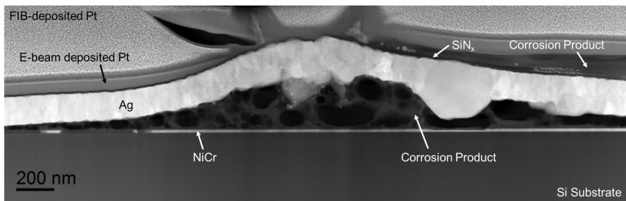
Figure 98. ADF image of cross-section of small corrosion feature on \text{NiCrN}_x adhesion layer mirror.
