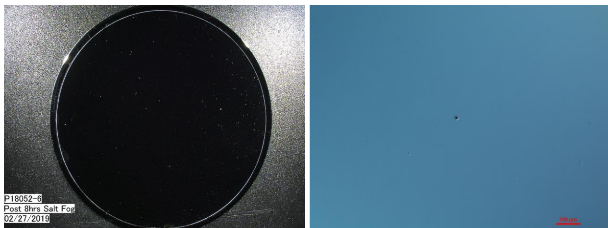
Figure 56. Dark field images of a NiCrN x adhesion layer mirror with corresponding optical micrograph of corrosion features after 8 hrs salt fog exposure.
