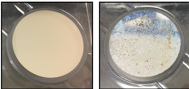
Figure 2. Freshly-deposited silver mirror (left) is smooth and reflective, compared to a degraded mirror (right) that is tarnished and corroded.
