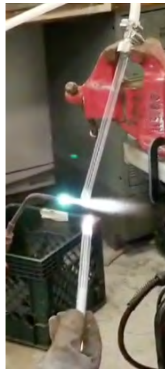
Figure 3.1: One may see the length of fused silica tube held in the quick connect, which is in turn mounted in the vise. The length of the glass tube used was not precise, but generally about 60 cm was desirable; much longer became unwieldy, and much shorter, about 30 cm or so, the flame became uncomfortably close to the sealing gasket, the samples, and the worker's hand.
