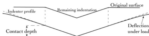
Figure 3.7: The material deflects around the indent. This must be accounted for in order to correctly calculate the indentation area. Original graphic after [113].
