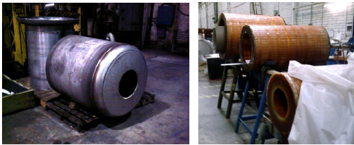
Figure 7. (Left) cryostat for 15-T solenoid; (right) coils for magnet. Coils are nested to produce the desired field.
