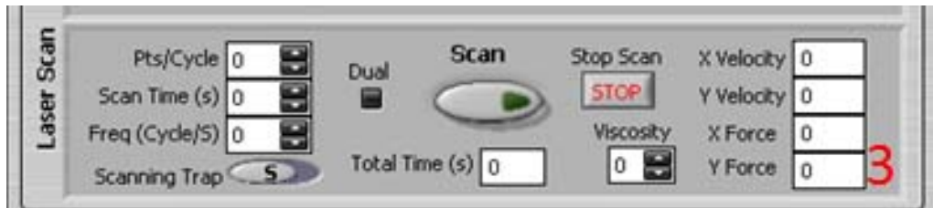
Figure B.8: Panel 3 Image showing control of the laser tweezers using laser scan
