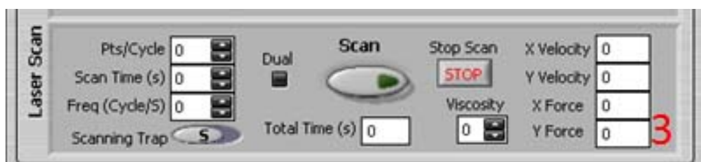
Figure B.4: Panel 3 is for dynamic control of laser tweezers
