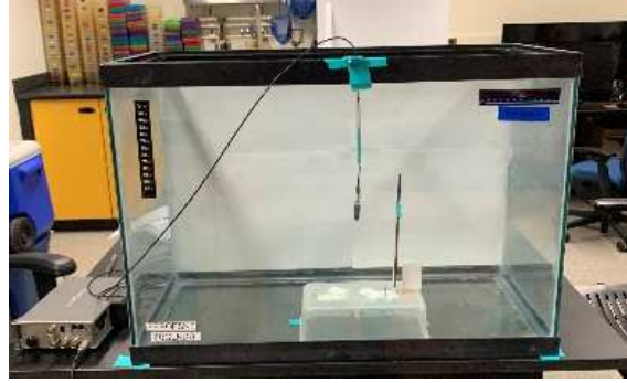
Figure 3: Shows the experimental aquarium, Sound Devices 277, and the Teledyne Reson tc-4301 attached to the Sound Devices 277 and hanging down into the experimental aquarium.
