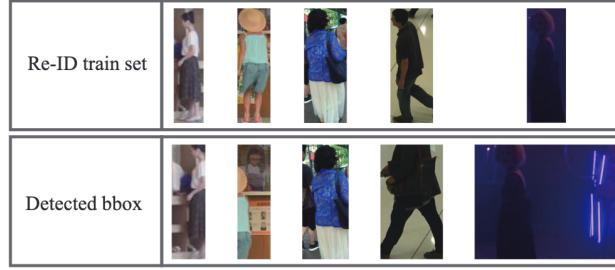
Figure 3.2: Demonstration of mismatch between ground truth and detected person bounding boxes. Figure from [121].
