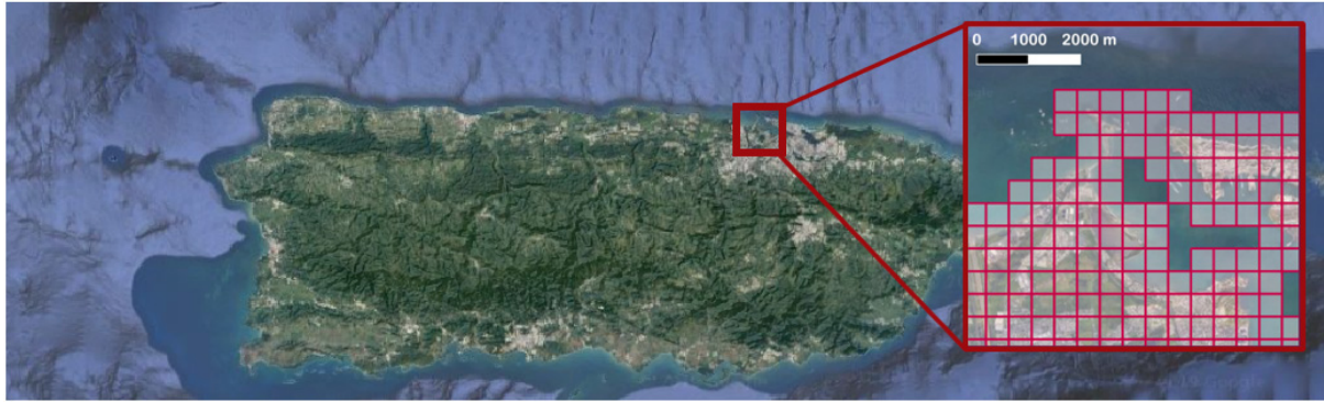
Figure 5. Zoomed-in view of the 500m meshgrid constructed across the island corresponding to VIIRS
