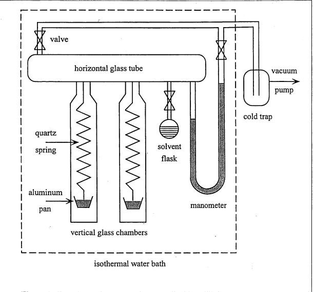
Figure 1 Experimental apparatus for vapor-liquid-equilibrium measurements
