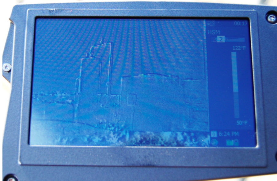
Figure 4: Filming a storage tank in Arvin, CA, above. Below, a close-up of the same tank on the FLIR camera's screen, shown in the infrared spectrum. Photo by author.
