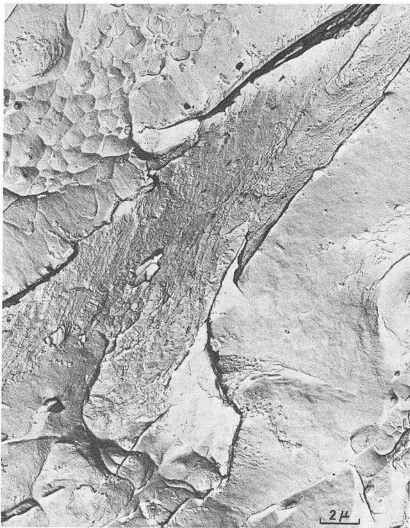
Fig. 4. Typical fractograph taken from a thick sample of B-450 materials tested at -196^{\circ} . (XBB689-5385)
