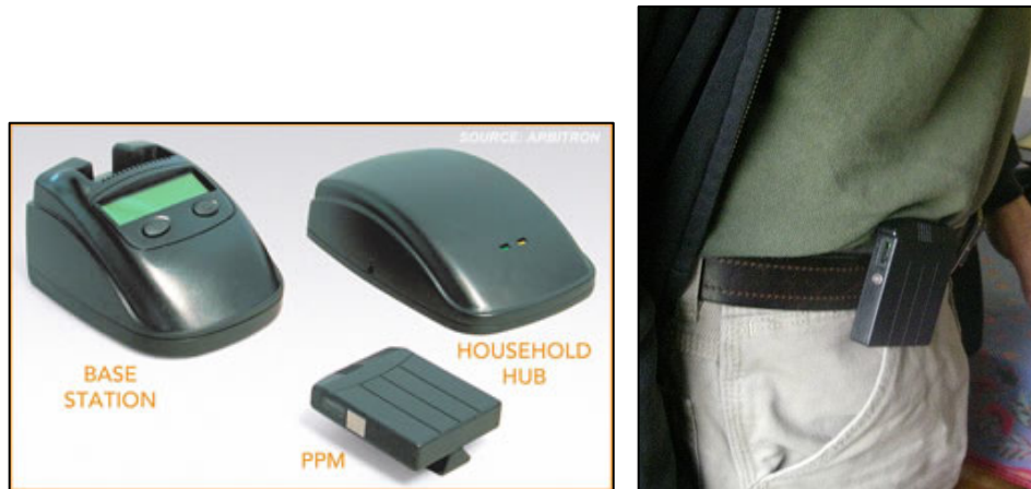
Figure 18: The three elements of the PPM technology: a base station, a household hub, and the PPM, which was designed for participants to carry with them or wear on their person 84
