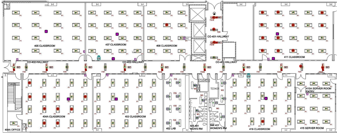
Figure 4.4: The layout of the fourth floor at the test site and the locations of the lighting fixtures and their integrated PIR occupancy sensors.
