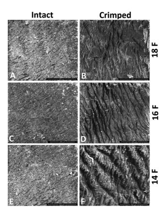
Fig 2. Scanning electron microscopy images show intact (A, C, and E) and crimped (B, D, and F) states of three different pericardial leaflets at 18F, 16F, and 14F, respectively. Comparison of scanning electron microscopy images demonstrates substantial changes on the surface microstructure owing to crimping, which increased with reduction of the collapsed profile.
