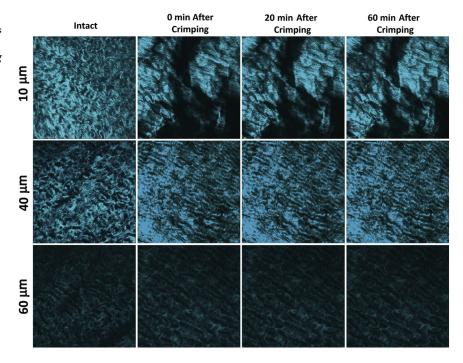
Fig 3. Second-harmonic generation microscopy images compare the structural changes of intact and crimped pericardial tissues at the depth of 10, 40, and 60  $\mu$ m for crimping size of 18F as a function of time.
