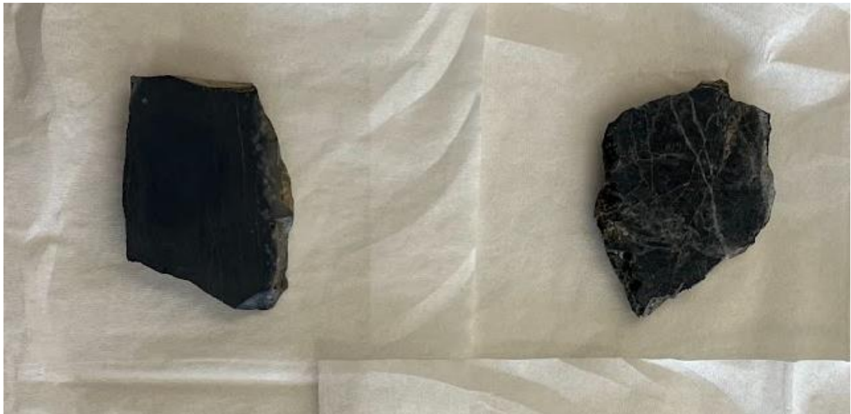
Figure 16 : Picture of two Union Wash samples, UW-12 (left) and UW-29 (right). Both samples show varying degrees of diagenetic alteration, with UW-29 displaying significant fracturing and re-cementation.
