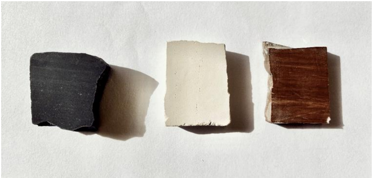
Figure 3: Photograph of three carbonate samples, prepared as 1-inch polished rock chips. Samples pictured display the range of colors present within the sample set. The oldest samples, i.e. Paleozoic, tend to be dark black to gray in color, similar to the leftmost sample below. Samples showing intermediate (brown, medium gray) and light (tan to white) colors only begin to appear in the Mesozoic.
