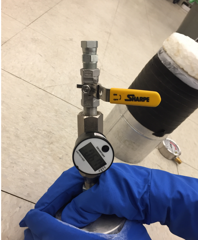
Figure 19 Pressure reading after inserting 30 mL of LN 2 and letting it completely evaporate inside of the vessel
