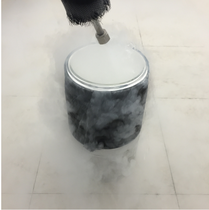
Figure 18 LN2 withdrawal from the LN2 reservoir to the transfer vessel
