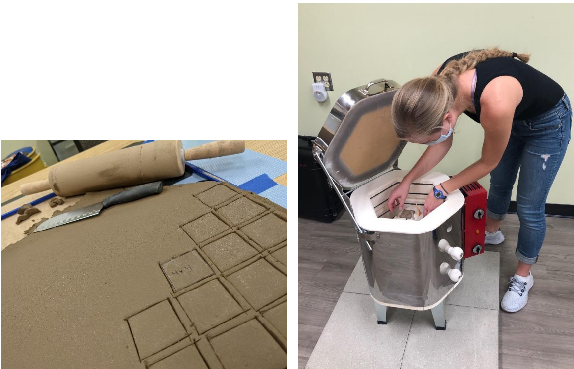
Figure 5 a & b: Rolled and Cut Out Clay Tiles (a) & Me Placing Tiles in the Kiln (b) (courtesy of Vanessa Muros)
