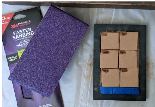
Figure 7: Image of Tile Abrasion Set-Up
