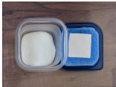
Figure 8: Image of Saturated Salt Container Set-Up
