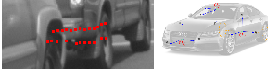
Figure 2.3: An example of parallax, caused by the distance between sensors. In this case, LiDAR is mounted on front bumper, and Camera is mounted behind the windshield.
