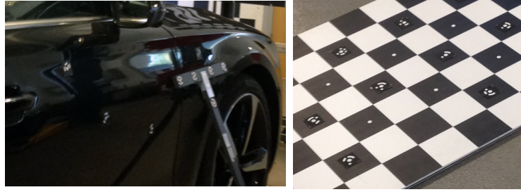
(a) Coded markers and T-shape scale bar (b) Checkerboard in front of the car
