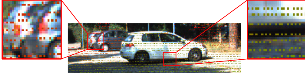
Figure 2.6: When LiDAR measurements are projected onto the image plane, they are roughly distributed evenly independent of their range.
