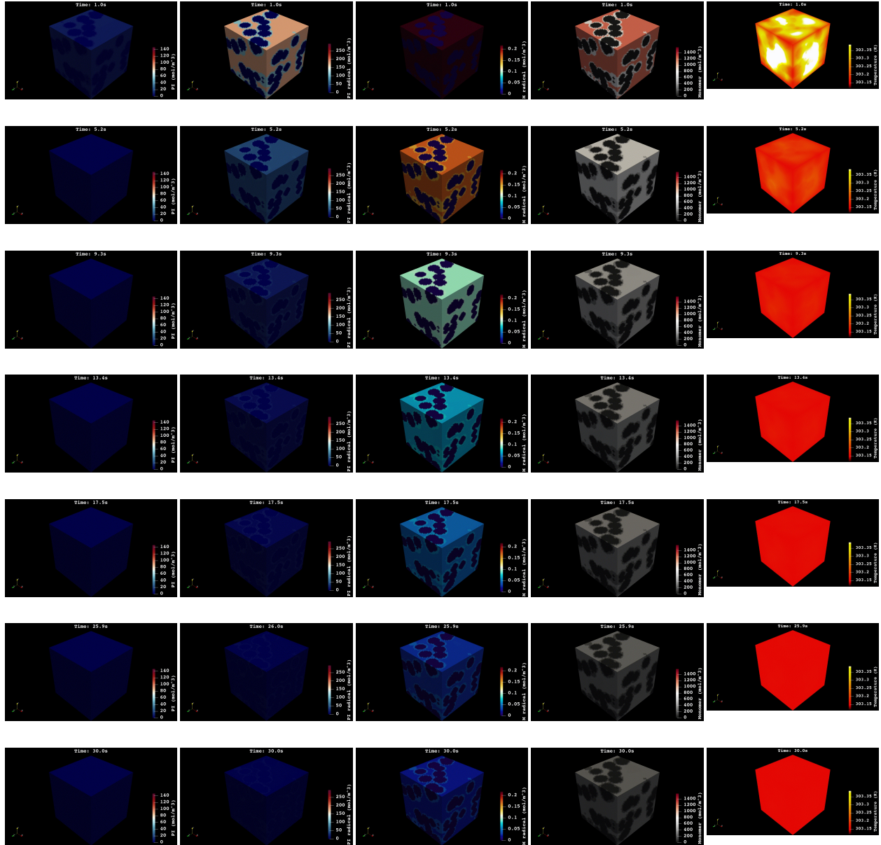
Figure 4.11: Dynamics of next 29s : Columns 1-5 show the time evolution of the concentration of PI, the primary radical ( \text{PI}\cdot ), the propagating radical ( \text{M}\cdot ), and the monomer ( \text{M} ), each with units \text{mol}/\text{m}^3 . The dynamics from 1-30s are dominated by the slower conversion of primary radical (column 2) to the propagating radical (column 3) to consumption of monomer (column 4). During this slower reaction phase, the convection to the surrounding environment provides a more stable temperature distribution.
