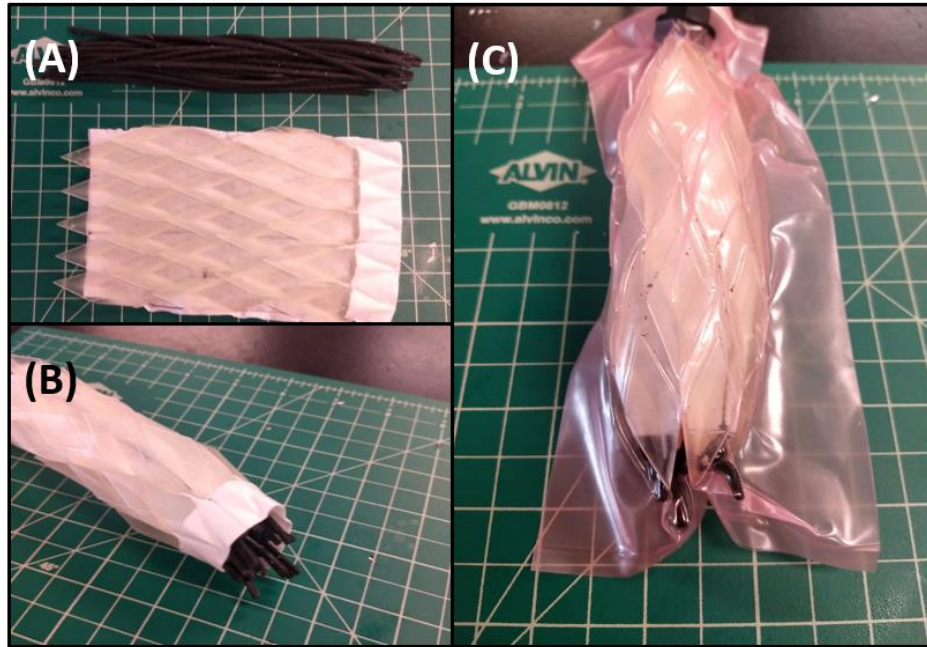
Figure 4.6 (a) Wires and ganoids can be assembled together (b) to form a tube with a wire core and a ganoid exterior. (c) The result is a jammer that can bend in any direction with high stiffness.
