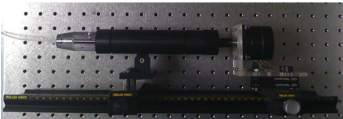
Figure 3.2: Fluidic setup of the microscope cell sorter. The CellTram Vario is shown coupled with a Vexa motor.
