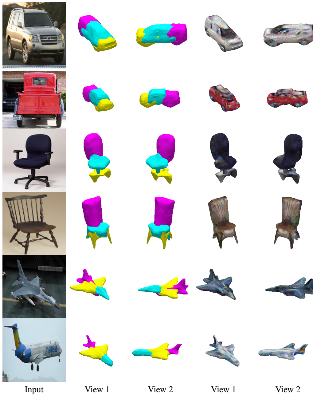
Figure 2.9: Part and color reconstruction results on the Pascal 3D+ dataset [132]. Despite that the dataset contains complicated 3D objects in a realistic scene, our method is able to discover consistent parts and effectively reconstruct the objects shapes.
