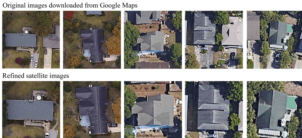
Figure 4.55: Comparison between original images from Google Maps and refined images produced by the roof segmentation model
