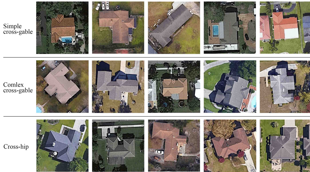
Figure 4.22: Example satellite images in testing dataset B (buildings with complex and mixed roof shapes)
