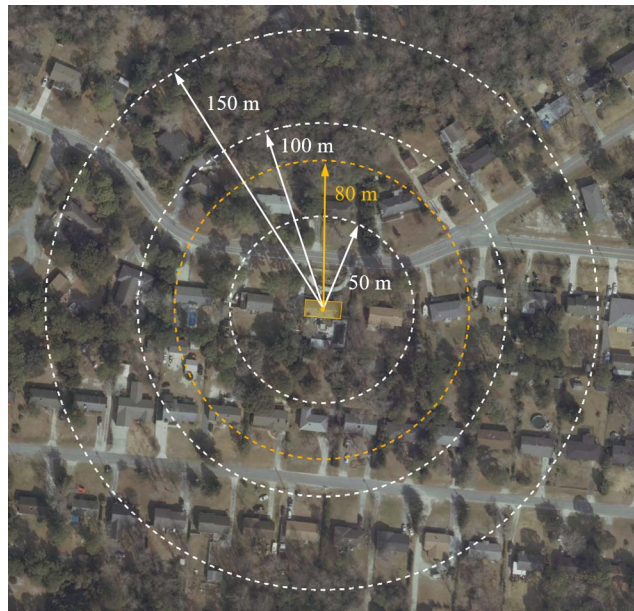
Figure 4.48: Candidate search radius used to calculate neighborhood-level roof type distribution for predicting missing roof-type data
