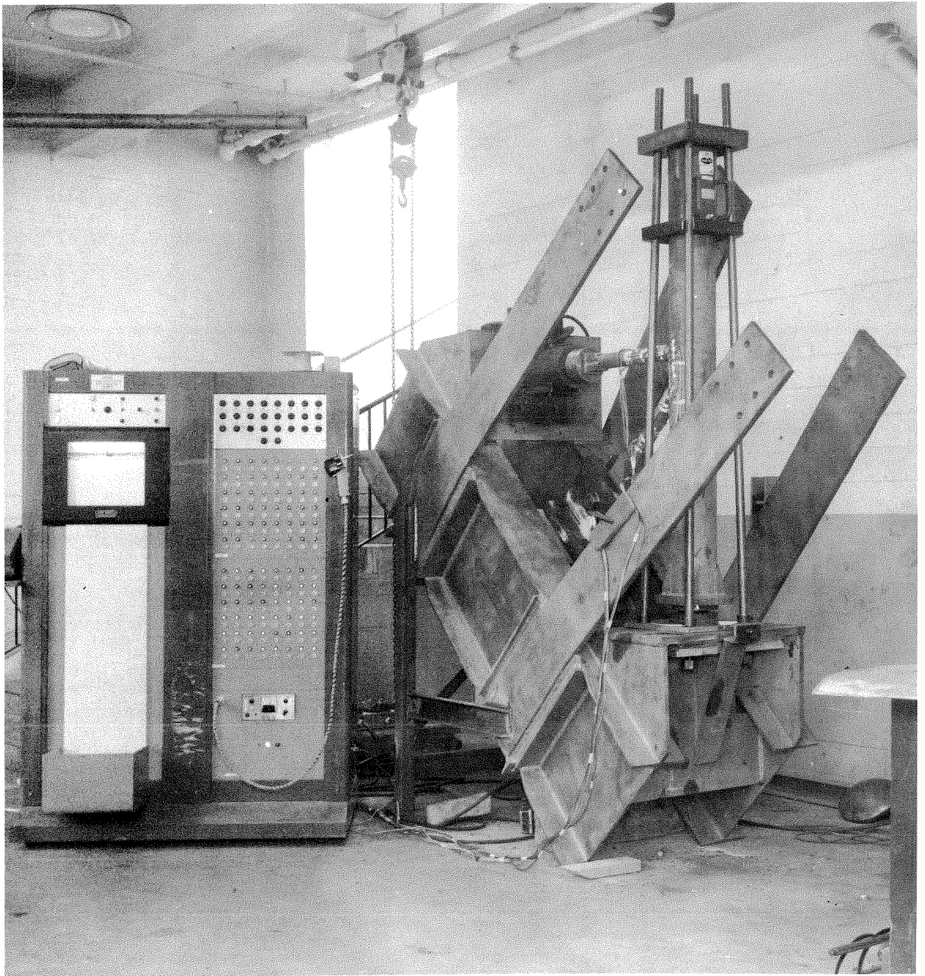
FIG. 12 LOADING FRAME AND RECORDING EQUIPMENT
