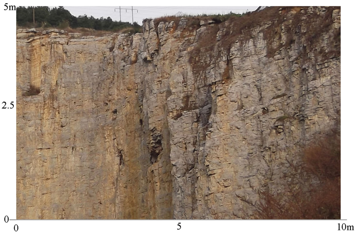
Fig. 4 Distribution of cracks and dissolution pores at the abandoned quarries A and B. the quarry profile was regarded as a soil reference level, and the soil leakage ratio was calculated as m/(n + m) , where
