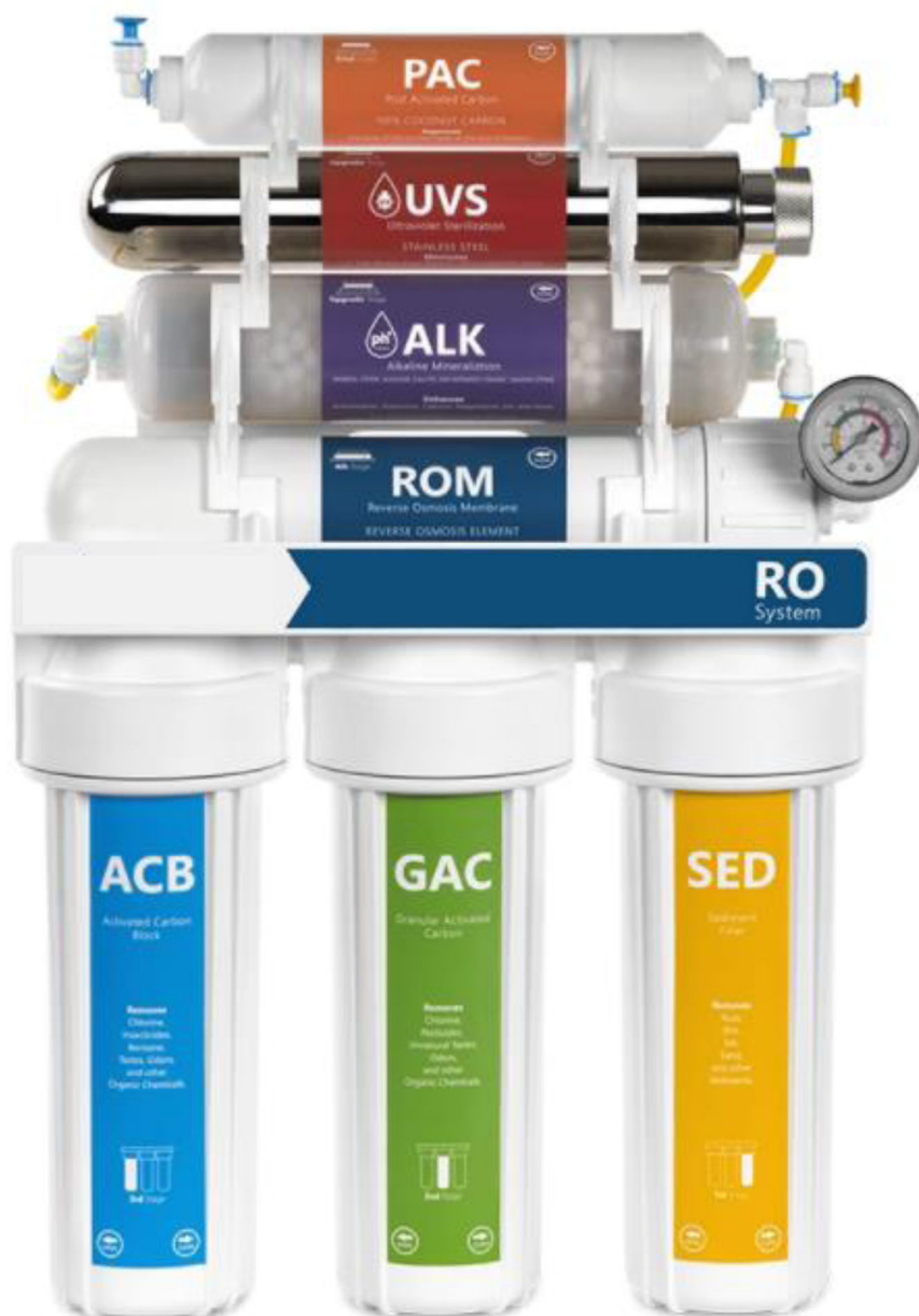
Fig. 8 Under-the-sink RO filtration. There is considerable flexibility in the number of stages depending on the needs of customers, which may contain up to seven stages including a sediment prefilter (SED), ion exchange (IEX), KDF or GAC media filters, activated carbon block (ACB) filters, RO membrane (ROM), remineralization media filters (ALK), UV sterilization (UVS) and/or postfiltration activated carbon (PAC) (reprinted with permission from 181 ; Copyright © Express Water Inc., 2020).
