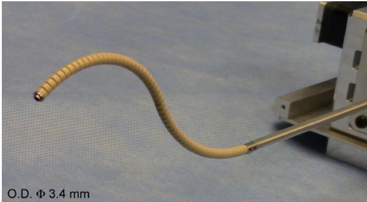
Figure 1.2. This figure, originally appeared in Takahisa Kato et al.[19], shows a tendon-driven robot with a diameter of 3.4mm
