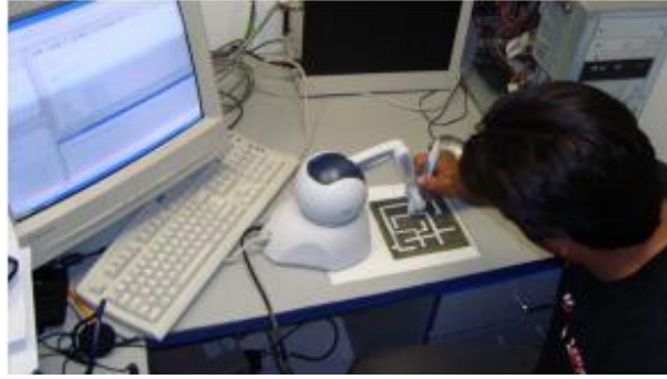
Figure 1.6. This figure, originally appeared in Bo Ouyang et al.[4], shows a Phantom Omni used as a input device.
