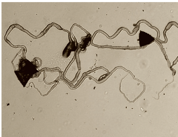
Fig. 14 Picture representing the transformation of crystals from their crystalline form to tubular formations upon addition of large cations to the aqueous solution in which the tubes are immersed.
