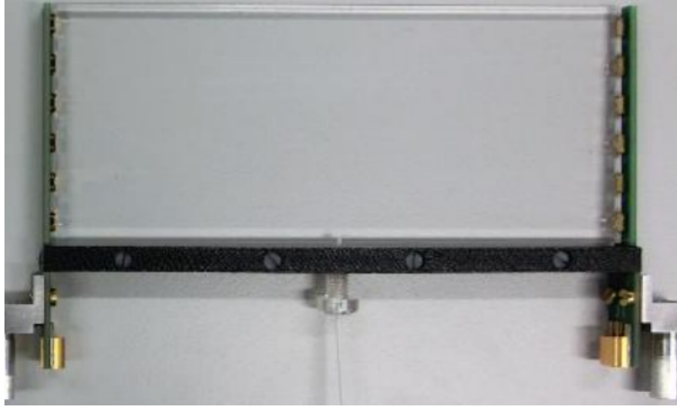
Figure 3.14: A single pixelated timing counter tile.
