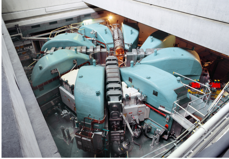
Figure 3.3: PSI's proton ring cyclotron.
