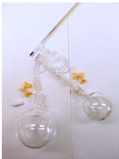
Figure 5-4: Distillation apparatus components and assembled setup.
