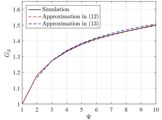
Fig. 2: Average throughput gain versus number of reconfiguration states. The parameters are  $\rho = 10$  dB,  $N_r = N_t = 17$ ,  $L_r = L_t = 5$ ,  $N_{\psi, cl} = 3$ ,  $N_{\psi, ry} = 10$ ,  $\sigma_{\theta^r} = \sigma_{\theta^t} = 4^\circ$ , and  $d/\lambda = 1/2$ .
