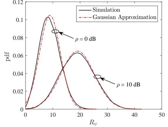
Fig. 1: Pdf of  $R_\psi$ . The parameters are  $N_r = N_t = 17$ ,  $L_r = L_t = 5$ ,  $N_{\psi, cl} = 3$ ,  $N_{\psi, ry} = 10$ ,  $\sigma_{\theta^r} = \sigma_{\theta^t} = 4^\circ$ , and  $d/\lambda = 1/2$ .
