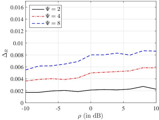
Fig. 3: Average throughput loss ratio versus transmit power to noise ratio. The parameters are  $N_r = N_t = 17$ ,  $L_r = L_t = 5$ ,  $N_{\psi,cl} = 3$ ,  $N_{\psi,ry} = 10$ ,  $\sigma_{\theta^r} = \sigma_{\theta^t} = 4^\circ$ , and  $d/\lambda = 1/2$ .
