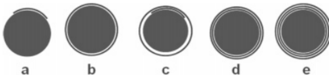
Figure 2.21: Illustration of the layer-by-layer encapsulation mechanism of catalyst particles. Atoms in the outer layers (a and b) may arise directly from carbon feedstock decomposition near the edge of the growing layer or from the precipitation of atoms in the metal-carbide particle, whereas atoms in the inner layers (c-e) originate from the metal-carbide. Reproduced from [42]
