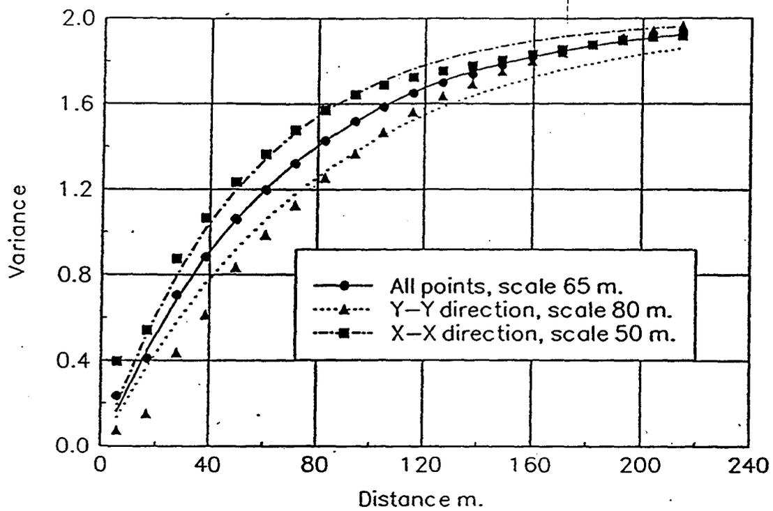
Figure 3. An experimental variogram of random anisotropic field.
