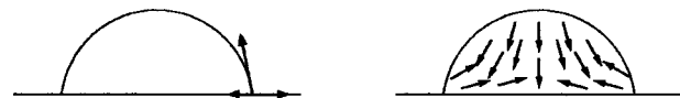
FIG. 14. The left diagram shows a force balance at the triple line only. This model cannot capture the effect of internal forces (shown schematically on the right) such as gravity or the forces due to internal electric fields. For example, the electric field of Sec. IV B, Fig. 4 will create forces everywhere inside the liquid.
